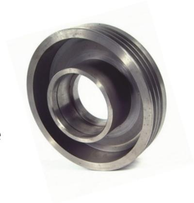
Dura-Bar ductile iron proved to be advantageous over steel for this pulley in the transportation and machinery industries. Many of Dura-Bar's advantages over low-carbon steel resulted in a significant cost savings for the customer. A key feature was Dura-Bar's superior machinability. The manufacture realized a cost saving because tool life was extended. Not only that, but an outstanding surface finish could easily be achieved with Dura-Bar.
