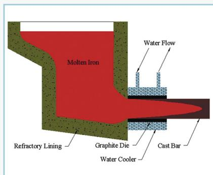
Above: Continuous Cast Bar Machine – Cross Section
