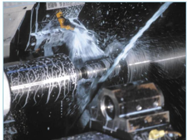
Above: Using continuous cast ductile iron in lieu of some free machining steels can save money by reducing machining cycle times by 25-50%.
