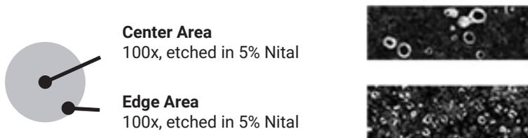
The microstructure consists of Type I & Type II nodular graphite as defined in ASTM A247. The matrix is highly pearlite with small amounts of ferrite. The edge or rim will have a higher nodule count and contain slightly higher ferrite concentration when compared to the center. Chill carbides will be less than 5% in any field at 100x and will be well dispersed.
