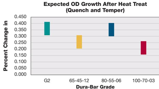
Data is based on 20 samples of each grade and the change in the outside diameter of a 1.00" machined specimen. All samples were heat treated to 1650° F, quenched in oil, then tempered to 450° F to a final hardness of Rc 50.
