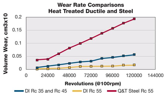
Data is based on 3 pad specimens on 52100 hardened steel disks, dry conditions, 150 lbs force.
