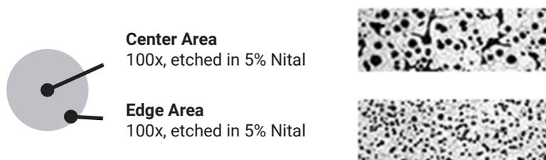
The microstructure consists of Types I & II nodular graphite as defined in ASTM A247. The matrix is ferrite with approximately 5-25% pearlite. The edge or rim will have a higher nodular count and will be mostly ferrite. Chill carbides will be less than 5% in any field at 100x and will be well dispersed.
